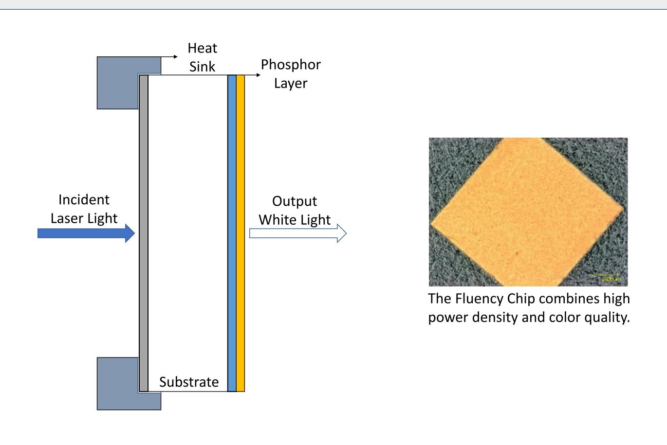
Due to high optical power density and high color quality, phosphor converted laser light sources hold great potential in applications that require focused, high intensity lighting.
