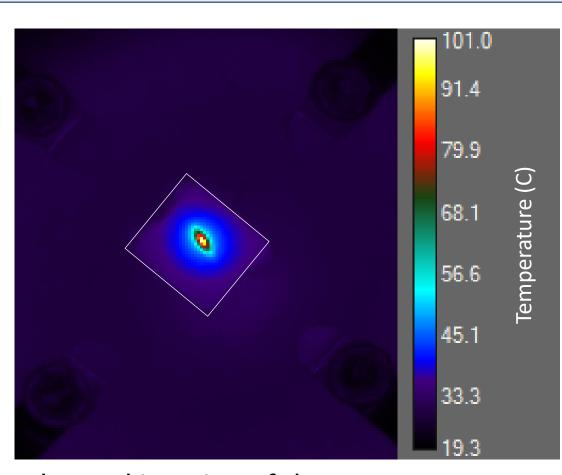
Thermal imaging of the converter.
