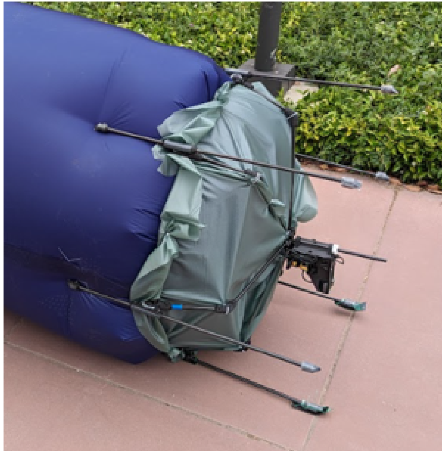
Figure 28: Image of the final tip mount design.
