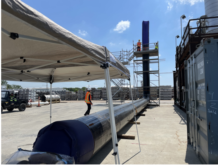
Figure 38: Vine robot body growth through the full pipe system without buckling was demonstrated.
