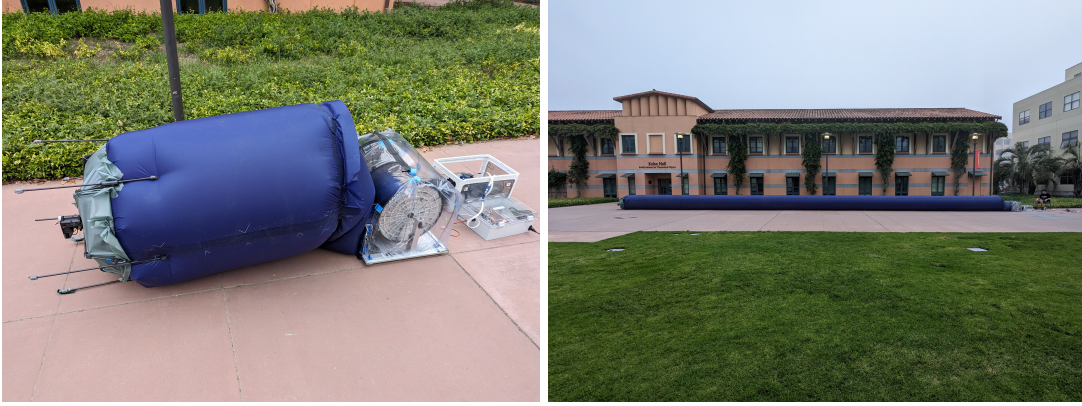
Figure 36: Base station with supporting subassemblies (left). Vine robot body grown to full length of 110 feet during testing at UCSB (right).
