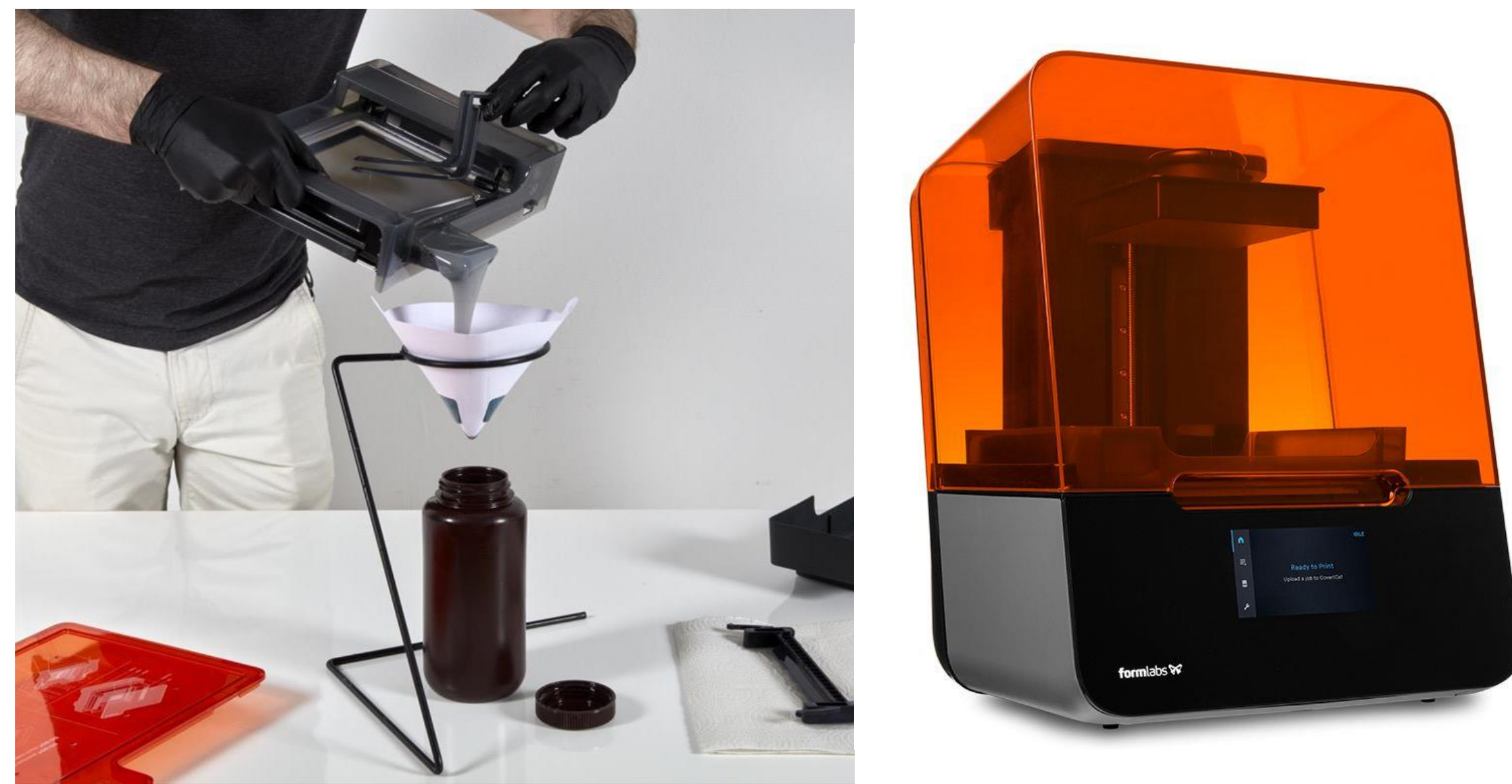
Figure 1. Formlabs SLA printers are frequently used for rapid prototyping and operate with a resin tank.
