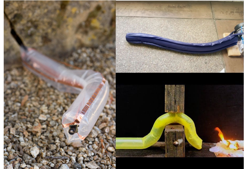
Fig. 1: Vine Robots can navigate cluttered and unpredictable environments. (Hawkes et. al., Coad et. al.)
