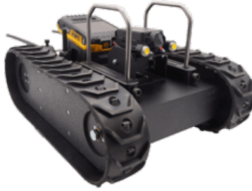
Figure 3: GPK-32 Tracked Wireless Inspection Robot.
